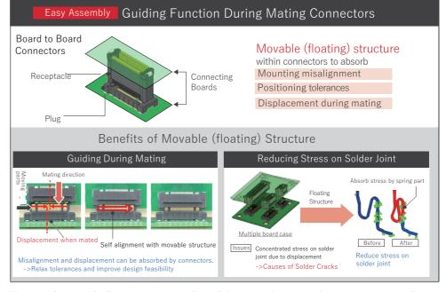
The main feature of a floating connector. Even if there is a slippage in the mounting or installation, the spring part in the connector will absorb the stress as long as it is within the movable range, which improves workability and reduces breakage.
