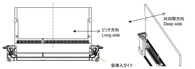
Insulator housing guide for the preliminary insertion
